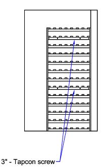
For uneven surfaces, like brick, we recommend using a slotted "L" bracket that you secure to the post with a 5/8" screw and then use a Tapcon screw to secure to the wall.
